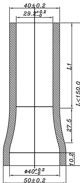
MODEL: MT-HTK011 Head Tube Material: Aluminum
